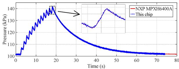
Fig. 10. Pressure measurement and comparison to a commercial sensor.
