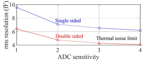
Fig. 8. rms resolution vs. ADC sensitivity when  $C_r = 5\text{pF}$ .
