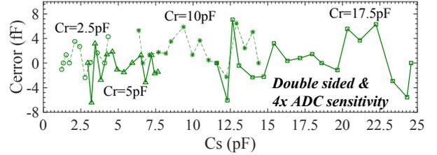
Fig. 7. Measured inaccuracy after 3-point calibration for various  $C_r$ .
