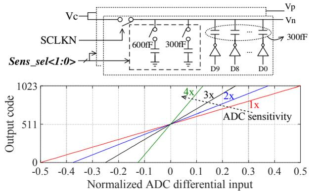
Fig. 3. Configurability of the ADC sensitivity.
