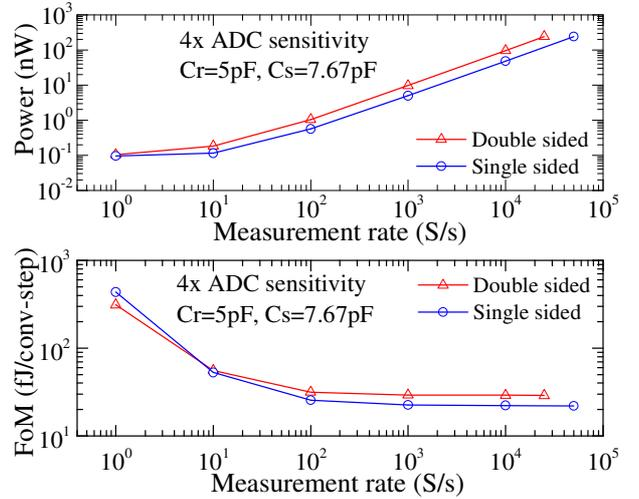
Fig. 9. Measured power vs. measurement rate (top), FoM vs. measurement rate (bottom) for  $C_r = 5\text{pF}$  and 4x ADC sensitivity.
