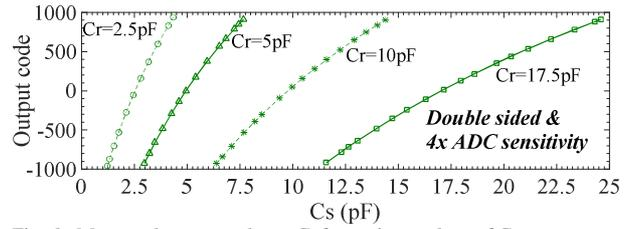
Fig. 6. Measured output code vs.  $C_s$  for various values of  $C_r$ .
