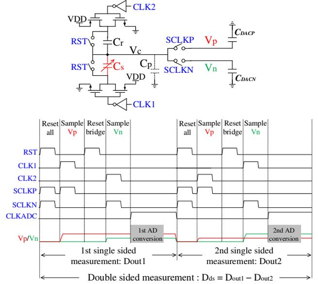
Fig. 2. Core of bridge and ADC (top) and operation waveforms (bottom).
