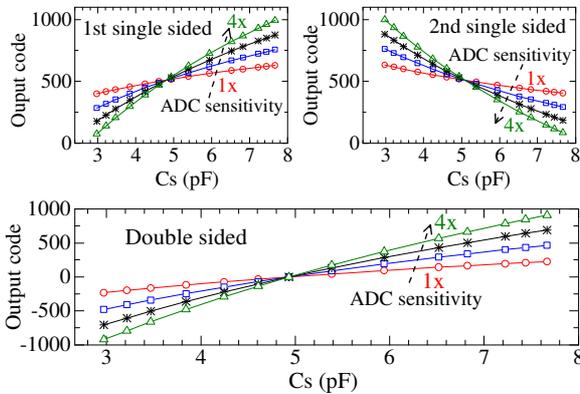
Fig. 5. Measured output code vs.  $C_s$  for various settings of ADC sensitivity when  $C_r = 5\text{pF}$ .
