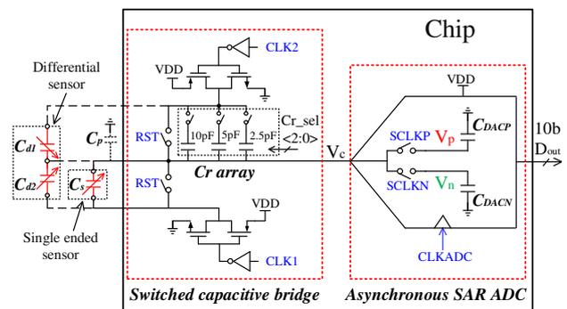
Fig. 1. Architecture of the versatile Capacitance-to-Digital Converter.
